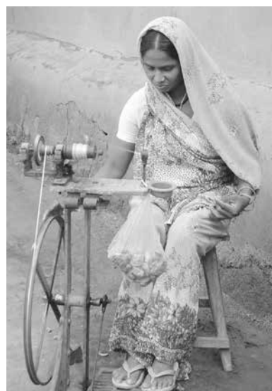
SHG member spins yarn from the pierced cocoons on the spinning machine in village Rajdah, Banka district, Bihar
