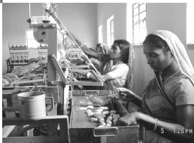
SHG members produce reeled yarn on a machine from the whole cocoons in Bhusitari Reeling Center, Banka district, Bihar.
