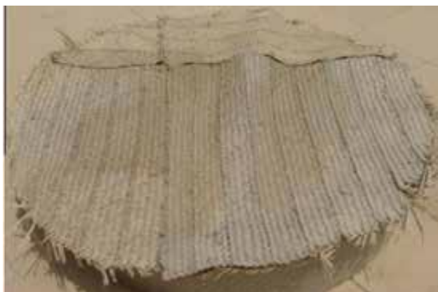
Photo 8: Example of palm fronds to cover ponds (Source: Alam, S., & AlShaikh, A. A. (2013). Use of palm fronds as shaded cover for evaporation reduction to improve water storage efficiency. Journal of King Saud University-Engineering Sciences , 25(1), 55-58)
