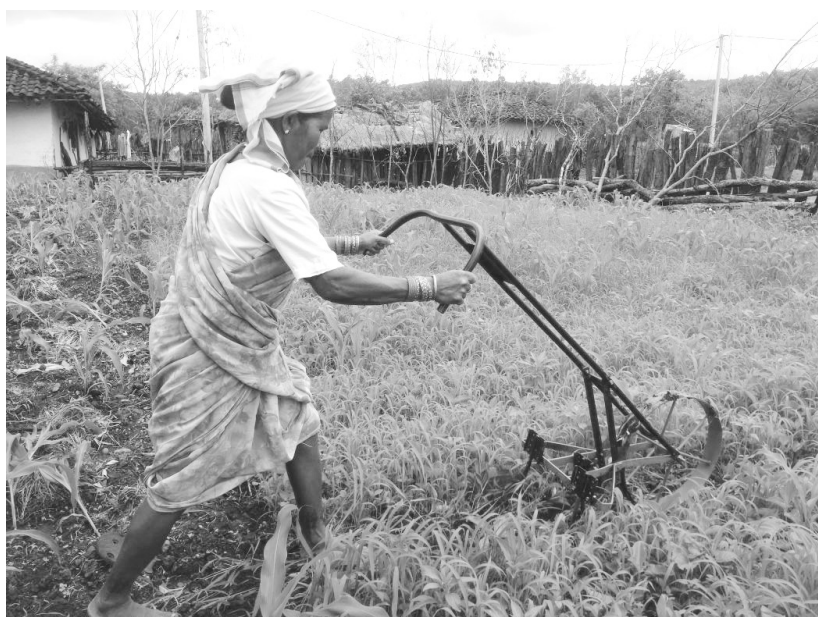
Kumhari Bai using weeder in her maize field, Gaura Kanhari village, Samnapur
